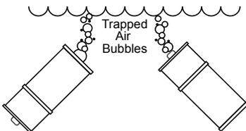
Submerge assembled filter in spa and tilt each end upward to remove trapped air bubbles from inside each filter cavity.
